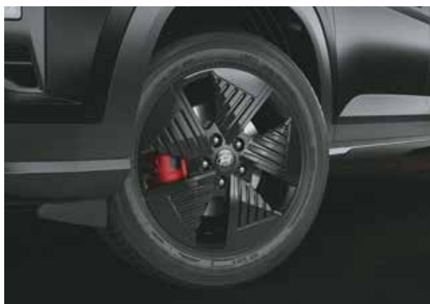
R17 (D=436.6 mm) Black aero alloy wheels with front & rear red brake callipers
