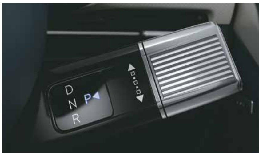
Shift by wire (SBW Column type)
