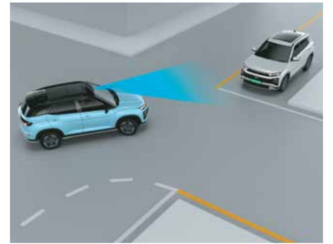
Forward Collision - Avoidance Assist - Junction Turning (FCA-JT) & Forward Collision - Avoidance Assist - Direct Oncoming (FCA-DO)
