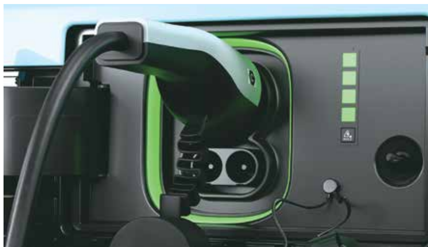
Charging port with multi-colour surround light and state-of-charge (SOC) indicator
